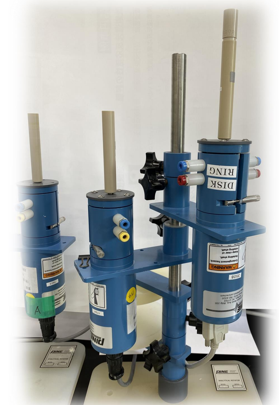
Potentiostat (Autolab PGSTAT128N). Electrode rotating device (PINE AFMSRCE)
